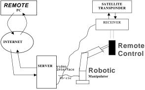
Figure 7: System Schematics
