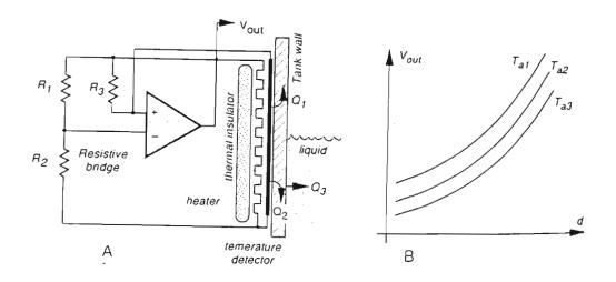
FIG. 3 - Active Thermoresistive Liquid Level Sensor
