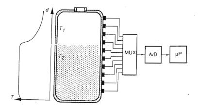
FIG. 2 - An Array Thermal Detector of Liquid Level
