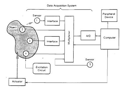
FIG. 1 - Positions of Sensors in a Data Aquisition System
