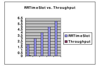
Since the round robin is the highest priority queue in the multilevel feedback queue scheduler, it has the greatest influence over the scheduler performance. With CPU Utilization of 80% and throughput of 0.024, time slot value of 4 time units comes out to be the optimal value in this simulation for the specific process mix.
