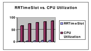
Figure 4. Charts illustrating effect of round robin quantum over performance measures
