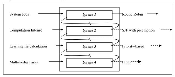
Another class of scheduling algorithms has been created for situations in which processes are easily classified into different groups/types. A multilevel queue-scheduling algorithm (see Figure 2) partitions the ready queue into several separate queues. The processes are assigned to a queue, generally based on some property of the process. Each queue has its own scheduling algorithm.
