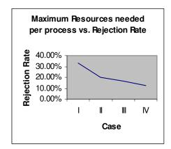
Table 12 shows the collected data and Figure 9 shows the corresponding graph. The statistics indicate that as the number of maximum resources needed for a process decreases so does the rejection rate. The total number of requests made is directly proportional to the maximum resources needed for a process. A decrease in the latter decreases the former and consequently decreases the rejection rate in a linear manner.
