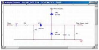
Figure 3: Phone detect circuit
