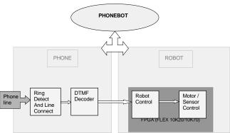
Figure 2: PHONEBOT - Basic Block Diagram
